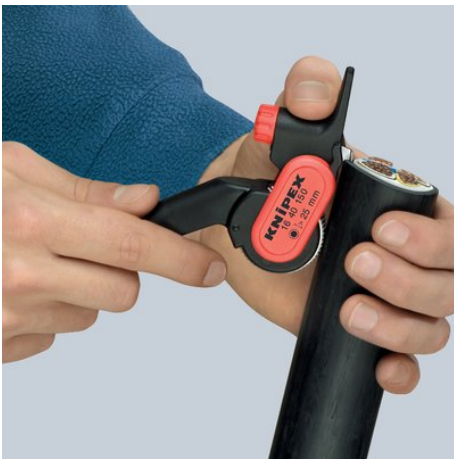
Setting the tool for longitudinal cut
