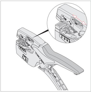
Readjusting the cutting depth
