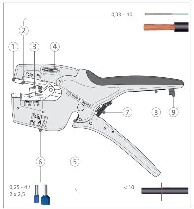
Structure of KNIPEX NexStrip®
