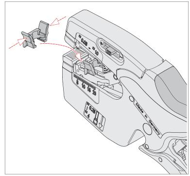
Replacing the feed stop
