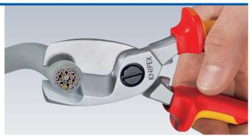
**Initial cut:** using the front cutting edge to cut the insulating sheath on larger cable diameters retains an ergonomic handle opening width.
