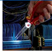
Multifunctional pliers for the electrical installation; to grip flat and round material, for bending, deburring, cutting cable, stripping and crimping end sleeves (ferrules)
