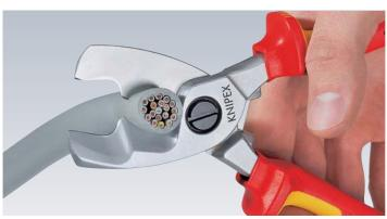
**Final cut:** after cutting the sheath in the front profile the conductors in the rear part are cut. Initial cut in the front profile, final cut in the rear profile - to keep it as easy as possible.
