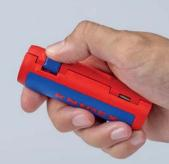
Convenient handling due to fastener with locking device and opening by means of internal spring
